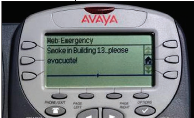
Avaya Broadcast Server telephone application allows reminders and alerts to be instantly distributed to displays of remote IP phones.
